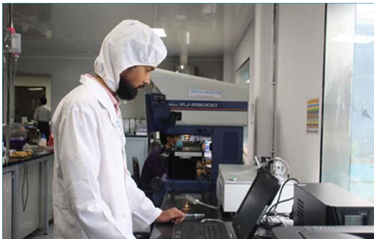
Needle Sharpness Test by Melab Measuring System, GmbH, Germany
