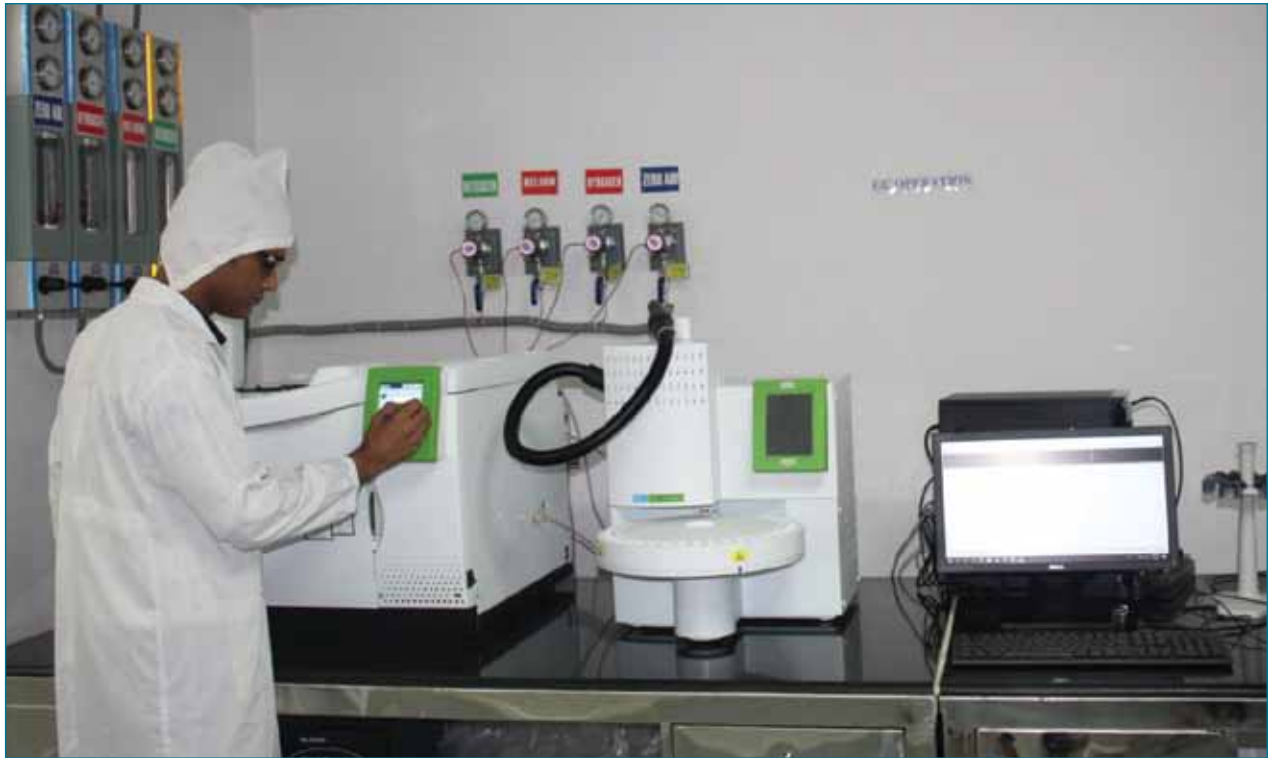
Picture: EO & ECH Residuals Content Test of Device Product by Gas Chromatograph (GC) Instrument-USA
